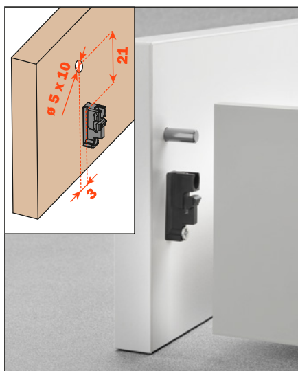
SMGP21X4XA Stabilizer pin 2-sided drawers, \varnothing 6 mm. Frontal drilling \varnothing 5 mm.
